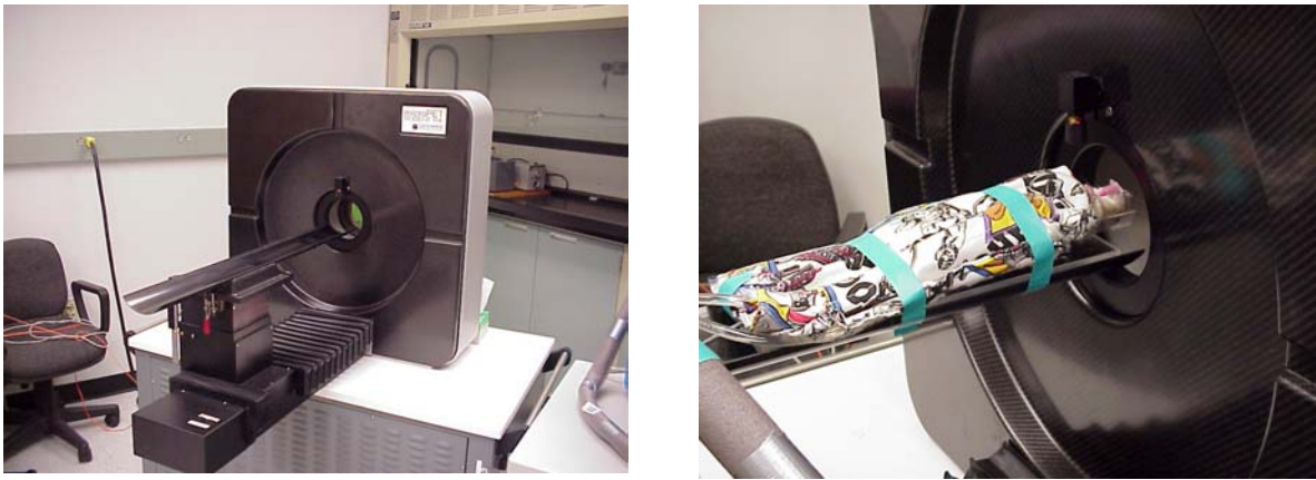
Figure 4: Photograph of the MicroPET system used to image oxygen-15. The picture on the right shows a rat that is covered with a water blanket for temperature control during imaging.
